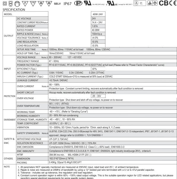
5. Derating may be needed under low input voltages. Please check the static characteristics for more details.
